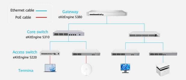
Based on the next-generation high-performance hardware and software platform, Huawei eKitEngine S220 series switches stand out with features such as flexible Ethernet networking, and diversified security control. In addition, eKitEngine S220 series switches support delivering higher performance and more powerful service processing capabilities. These make them ideal for various application scenarios, such as enterprise campus access and gigabit to the desktop.
