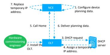
OLT ZTD builds a zero touch provisioning PON network to implement PnP and automatic deployment of network devices.
