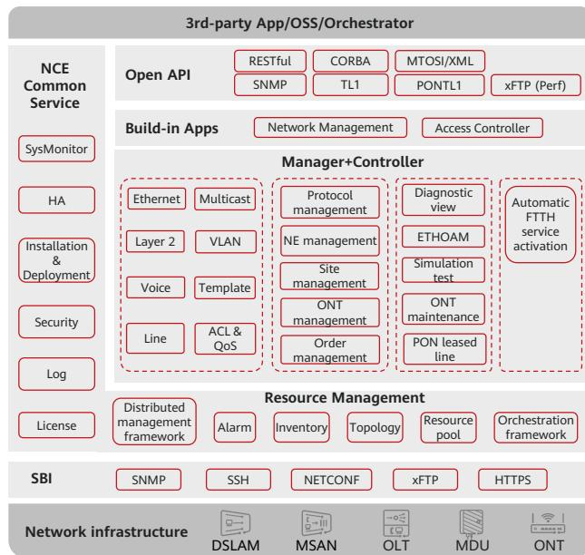
**Common service module:** provides basic network services such as alarms and logs and product engineering capabilities such as disaster recovery (DR) and backup.
